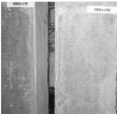
Fig. 10. Surface finish of the CPF faces of two of the test specimens (20% RHA and 15% RHA).
