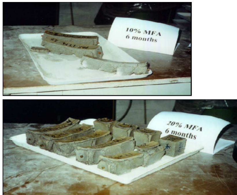
Fig. 6. Typical failure mode of mortar prisms and cubes.
