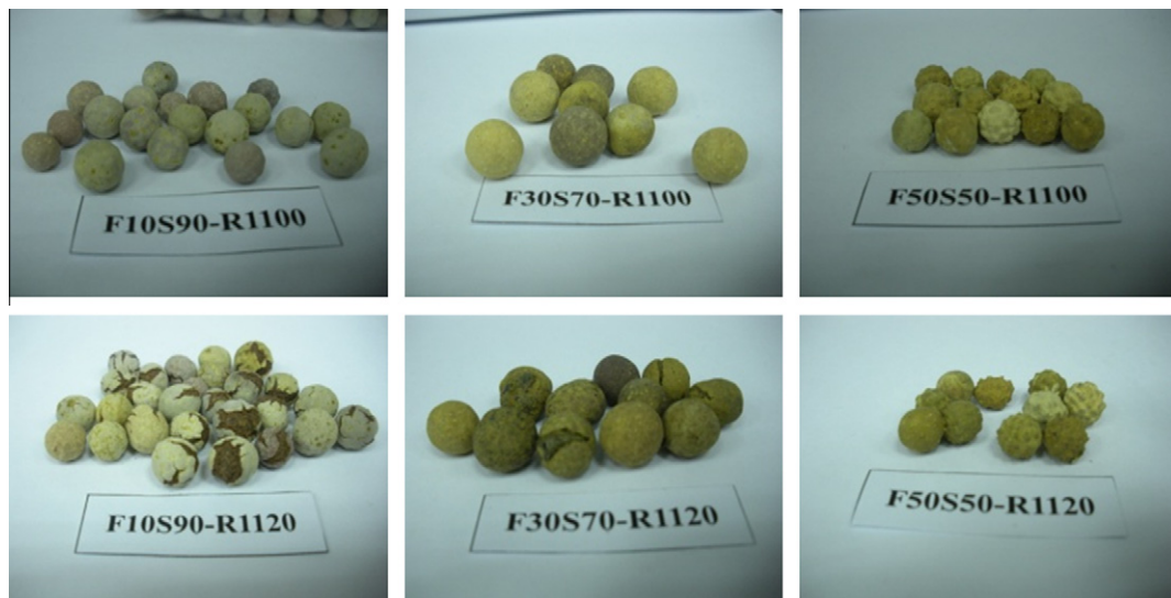
Fig. 3. External appearance and surface texture of produced LWA at 1100 °C and 1120 °C.
