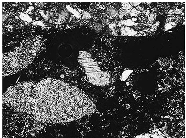
Fig. 6. In the center, a sodium plagioclase embedded in the calcium carbonate cement (dyed red), surrounded by fragments of visibly altered metamorphic rock. The rings are the result of the reaction between the rock and the carbonated paste.
