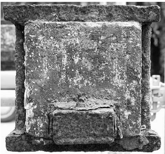
Fig. 2. Photography of anchorage device for prestressing steel wires.
