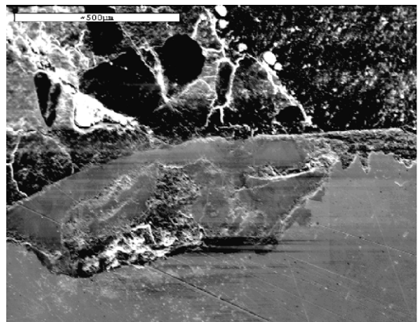
Fig. 19. SEM photography of steel/concrete interface for Sample B — Loc.2 (high-corrosion level).
