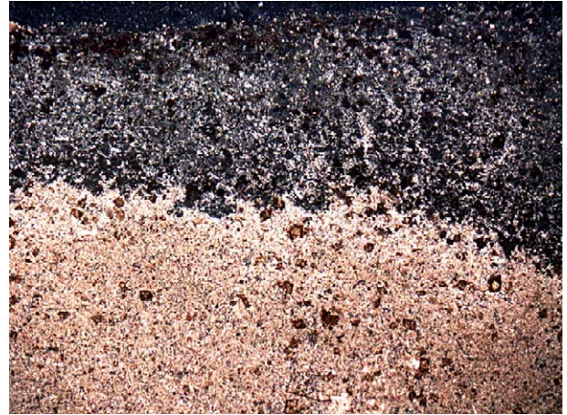
Fig. 16. LX aggregate after 28 days in LiOH 1 M. There is a significant alteration with partial carbonate alteration. It shows an alteration rim of 1.5 mm with external iron oxide rims near the borer. Cross-polarised light, horizontal field of view 5 mm.
