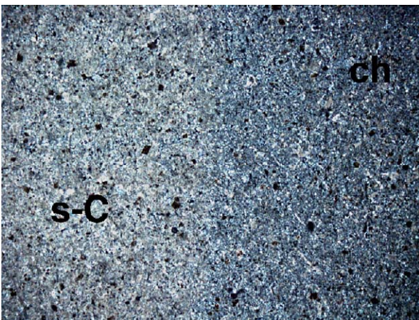
Fig. 4. The micrograph shows a limestone intensely silicified on the left part (s-C), and a micro- and cryptocrystalline quartz with calcite remains on the right (ch). Boundaries between the tow parts are not clear with diffused band. Cross-polarised light, horizontal field of view 5 mm.
