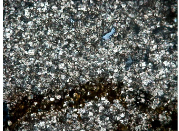
Fig. 2. Sucrose dolostone with coarse subhedral (planar-s) dolomite with slight zonation. Iron oxides are relatively abundant in all the samples, which tend to be located in bands. Cross-polarised light, horizontal field of view 1.25 mm.
