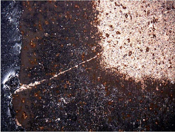
Fig. 15. CDX aggregate after 28 days in LiOH 1 M solution. Iron oxide is concentrated in the centre of the chert and just at the border. Cross-polarised light, horizontal field of view 5 mm.
