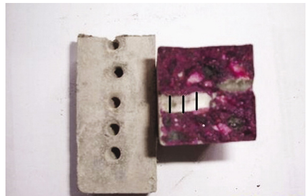
Fig. 1. Drilled concrete specimens for evaluation concentration of chloride at different depth intervals.
