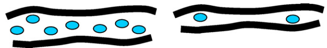
Fig. 1. The interlayer space is full on the left and empty on the right. Irregularities that cannot collapse further contain water in the IGP space. When this water is removed the IGP porosity remains (no further collapse), and it is the first space where water reenters upon rewetting.
