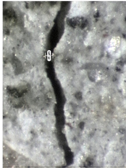
b) \text{COD}_{\text{max}} = 105 \mu\text{m} , w_1 \approx 35 \mu\text{m}
