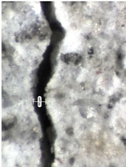
c) \text{COD}_{\text{max}} = 154 \mu\text{m} , w_1 \approx 50 \mu\text{m}
