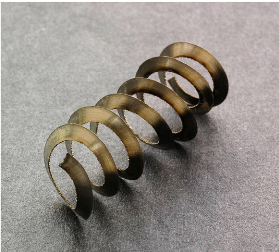
Fig. 1. A helix-shaped support on which the cement paste samples were applied.
