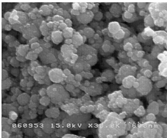
Fig. 2. Scanning electron micrograph of \text{Ce}_{0.8}\text{Gd}_{0.20}\text{O}_{1.90} powder prepared by microwave-induced combustion.
