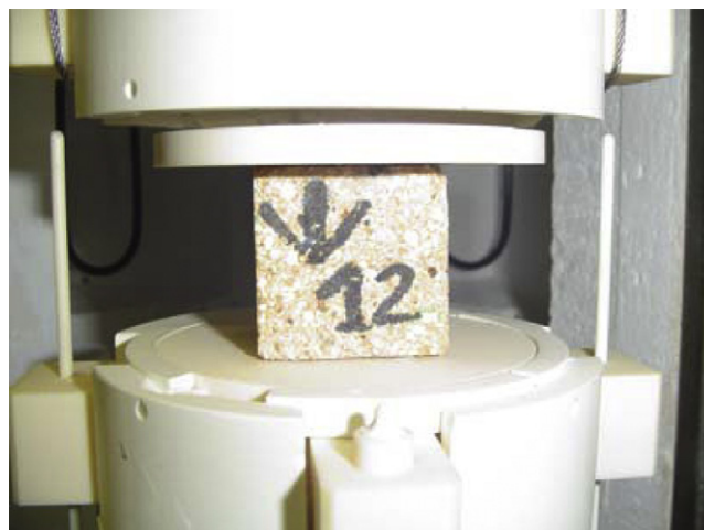
Fig. 2. View of a prefired BSAA sample in the uniaxial compression set-up during the preparation phase.
