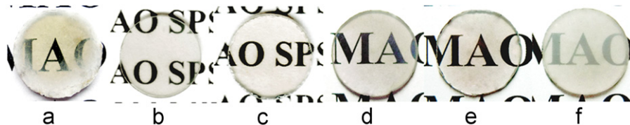
Fig. 4. Optical transparency of MgAl 2 O 4 sintered at different temperatures for 20 min: (a) 1250 °C, (b) 1275 °C, (c) 1300 °C, (d) 1325 °C, (e) 1350 °C and (f) 1375 °C.
